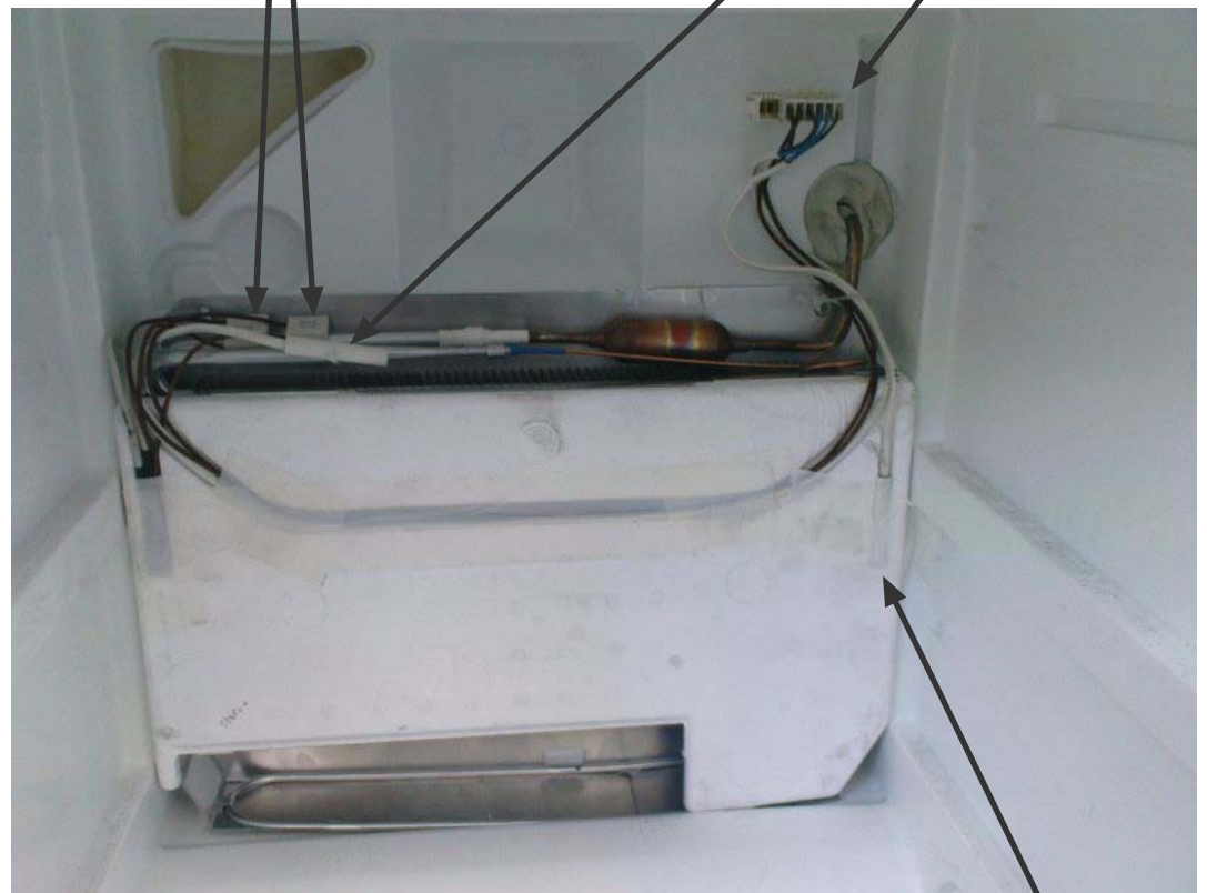
Not restorable thermofuses with integrated defrosting sensor.
