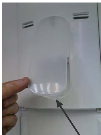
Lamp cover removing: open this side
