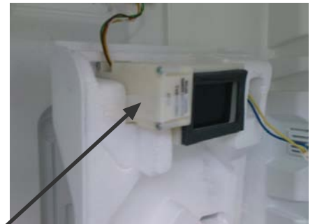
Fixing Adhesive strip for damper element
