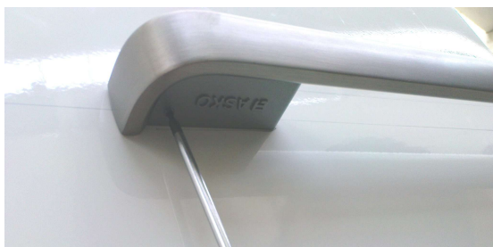
3 - Unscrew at the lower side
