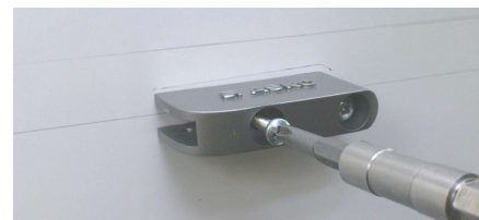
6 - remove the handle support
