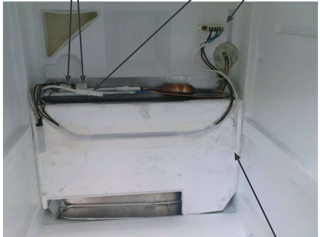
Not restorable thermofuses with integrated defrosting sensor.
