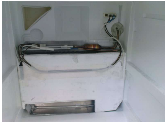
No frost radiator view in the freezer compartment
