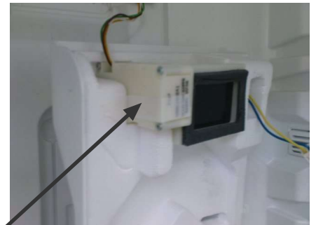
Fixing Adhesive strip for damper element
