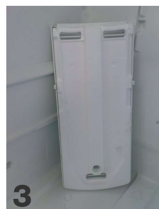
Lower diffuser part internal insulating
