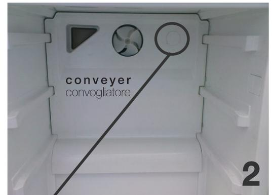
2- Once removed the conveyer cover we can see the conveyer: (pic. 2)
