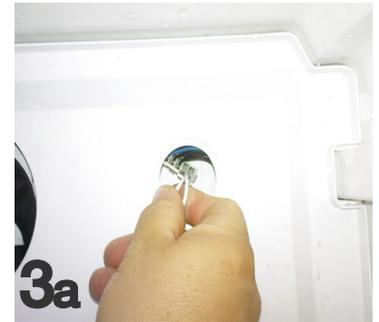
3a - Remove the fan connector at right side
