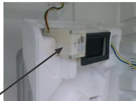
Fixing Adhesive strip for damper element
