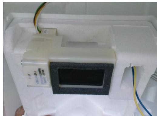
Before to close the diffuser we can make sure about the right functioning of the damper by switching on and off the only fridge compartment on the control panel by reading the instructions on the hand booklet of the product.
