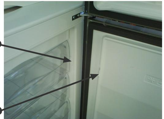
**Note: Both reed and magnet for freezer compartment are only available on display model**
