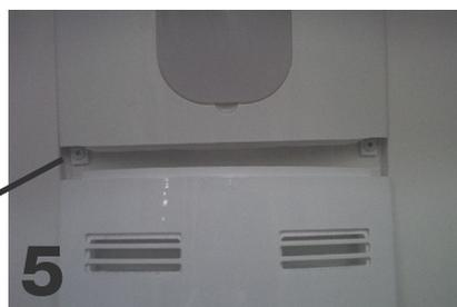
**5 - when removing the lower diffuser part we can see the fixing screw for the upper part diffuser.**
