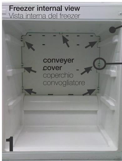
1 - Air diffuser fixing hooks pressure mounted
