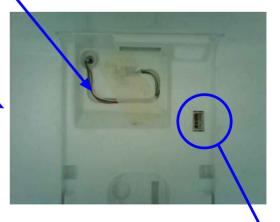
New wiring integrated in the foam for the lamp connection
