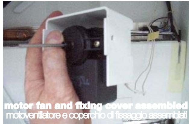
Place the motorfan plastic pin inside the hole on the rubber gasket of the motorfan support and then assemble the motorfan box to the conveyer by inserting the steel pin on the related place on the rubber support placed on the conveyer.
