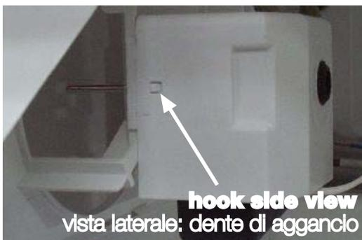
After have removed the box, extract the motor fan: older models provided with back side connection have the motorfan connector connected to the back side module while, instead, the newer models have the motorfan connector connected to the internal connector. Find the related connector according to the wiring diagram of the appliance we are repairing.
