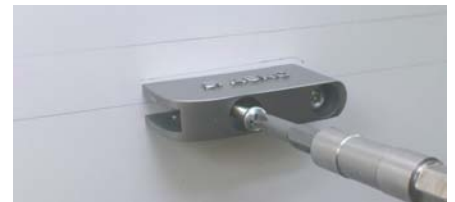
6 - remove the handle support
