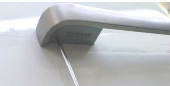
3 - Unscrew at the lower side
