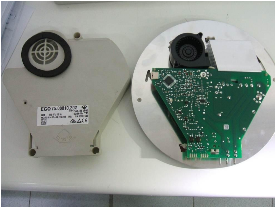
Induction generator module; 75.08010.202 – external bottom view and PCB
