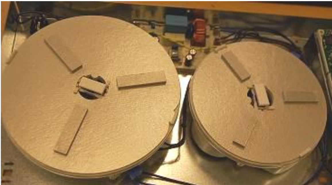
Induction generator modules; 75.08010.202 (left), 75.08010.102 (right)
