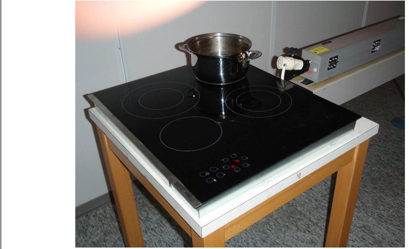
Notes: Test set-up for Disturbance Power
