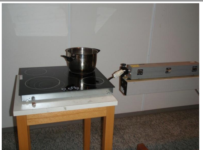
Notes: Test set-up for Disturbance Power
