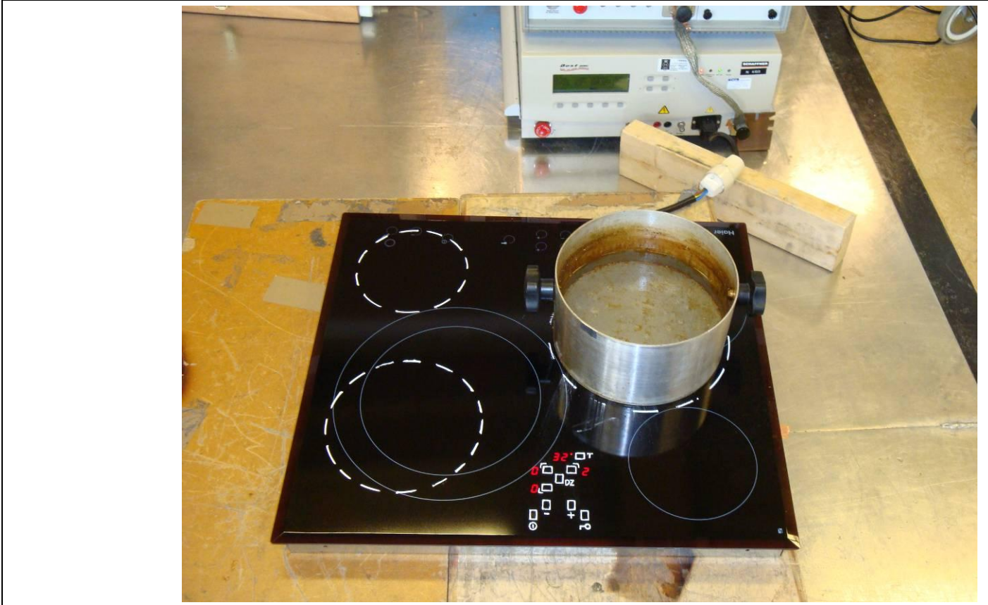
Notes: Test set-up for Electric Fast Transients, Surge and Voltage Dips
