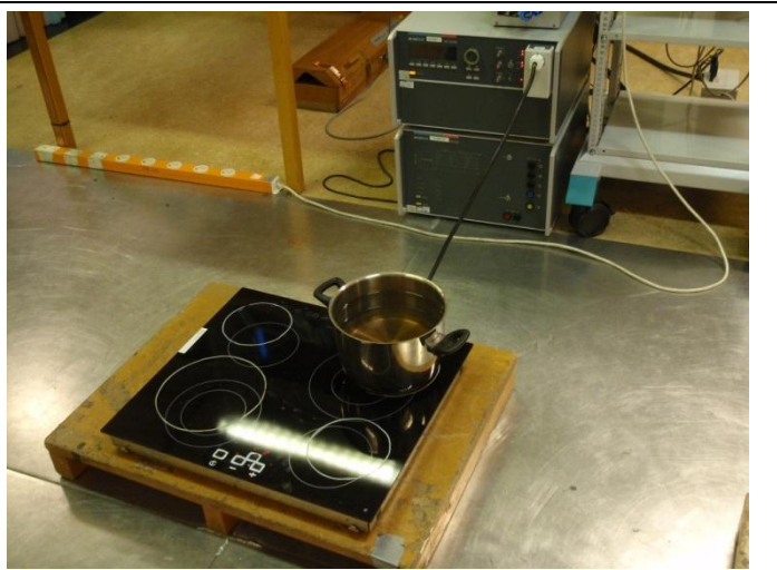
Notes: Test set-up for EFT and Surge
