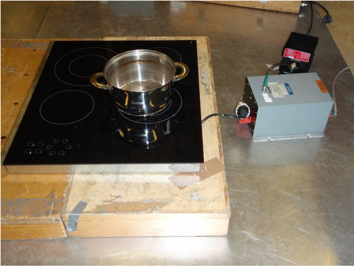
Notes: Test set-up for Conducted RF Disturbance
