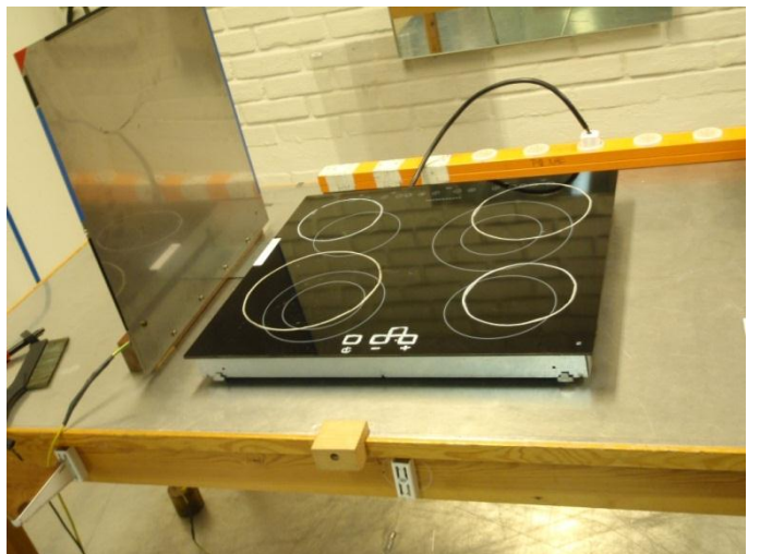
Notes: Test set-up for immunity to ESD
