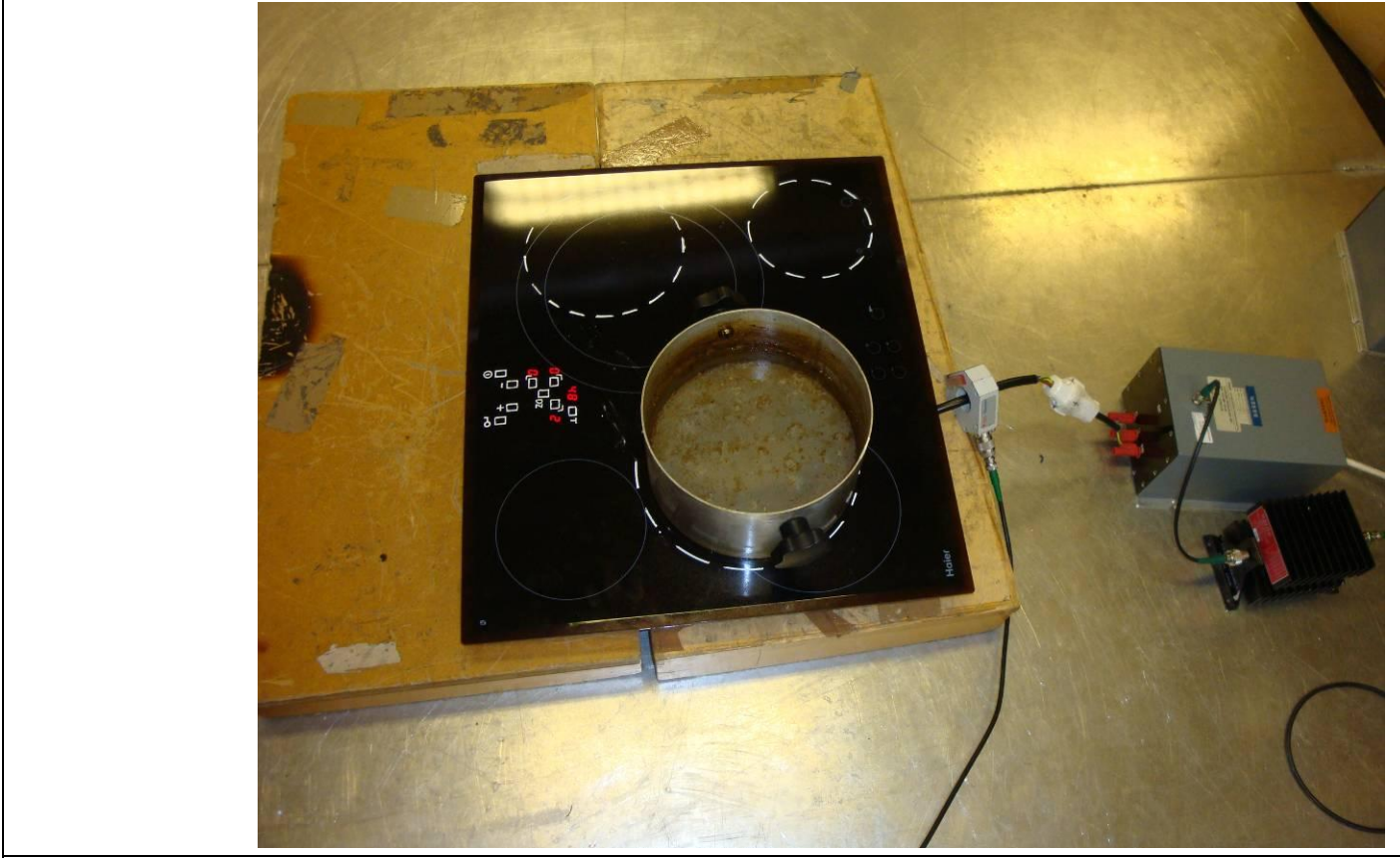
Notes: Test set-up for Conducted RF Disturbance
