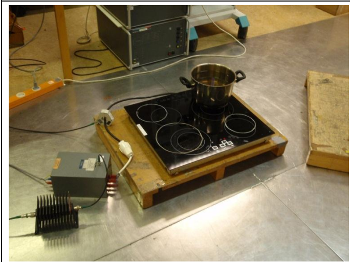
Notes: Test set-up for Injected current
