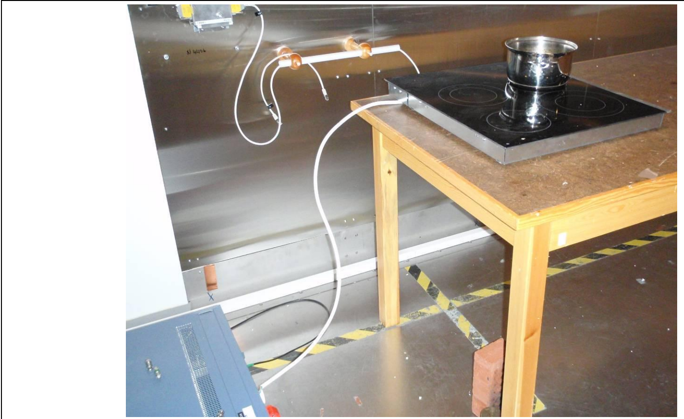
Notes: Test set-up for Mains Port Disturbance Voltage
