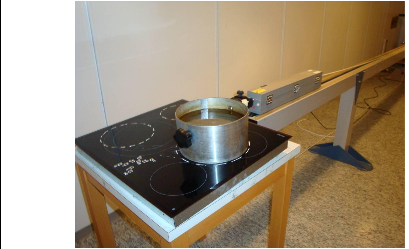
Notes: Test set-up for Disturbance Power
