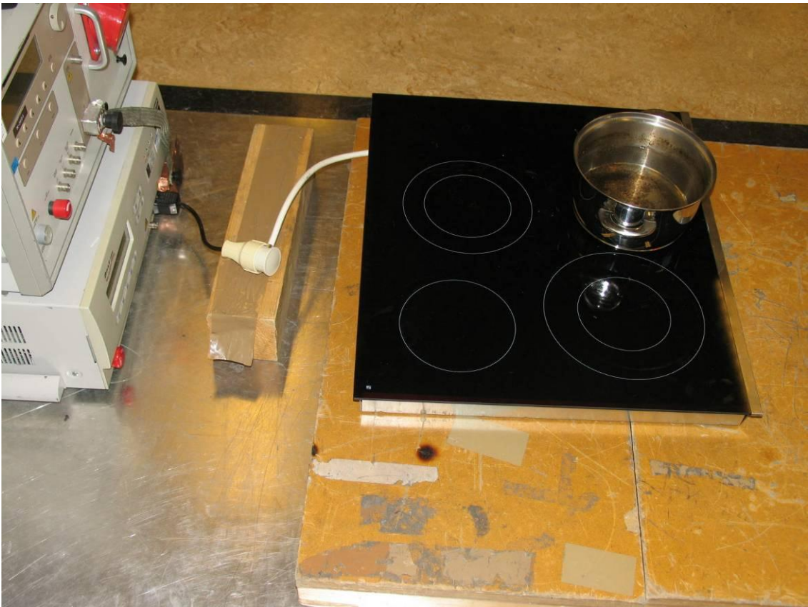
Notes: Test set-up for Electric Fast Transients, Surge and Voltage Dips
