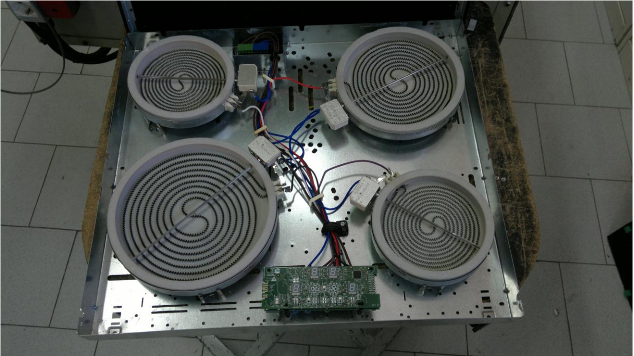
New control PCB BN340D36211107 in EO6400
