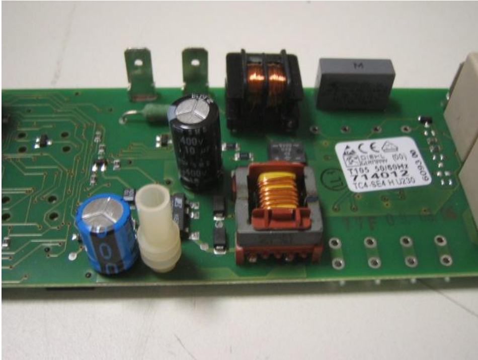
DIEHL electronic board: transformer side.
