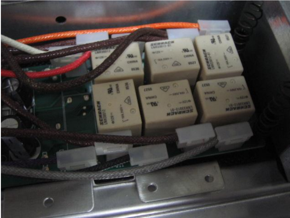
Relays on EIKA electronic board
