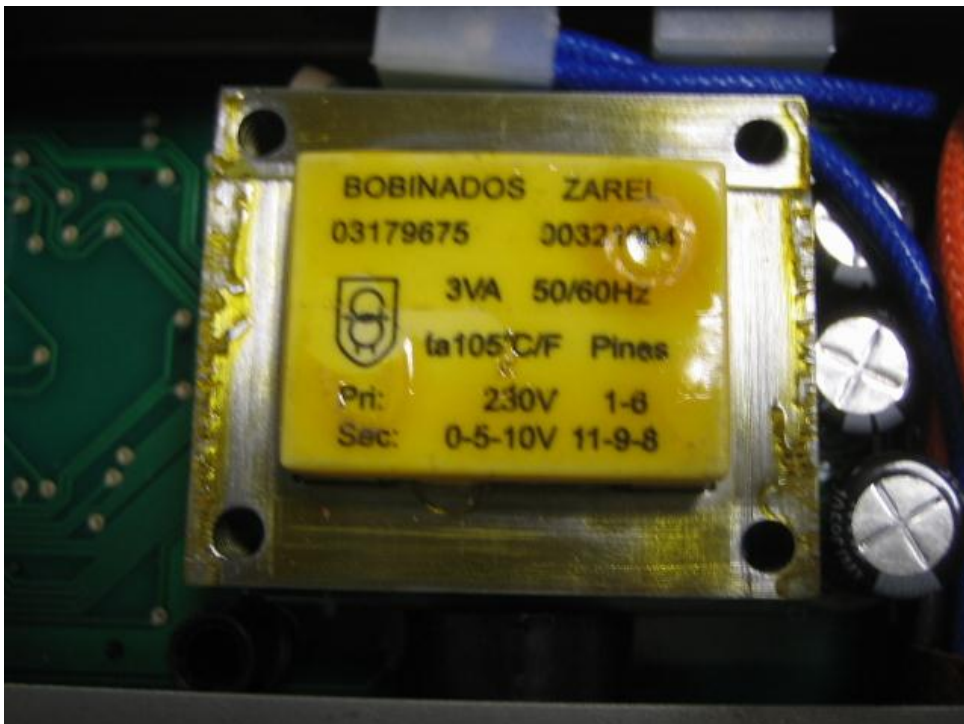
Transformer of EIKA electronic board
