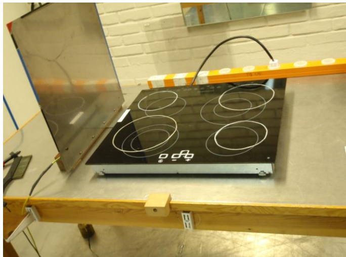
Notes: Test set-up for immunity to ESD
