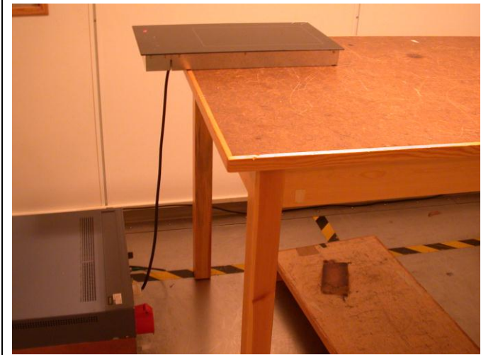
Notes: Mains Port Disturbance Voltage
