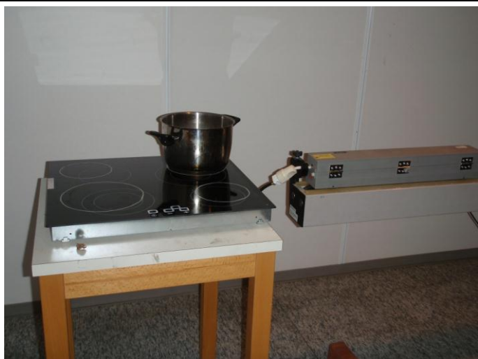
Notes: Test set-up for Disturbance Power
