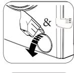
• You may use the washing powder spade supplied with your machine or liquid detergent level plate to open the pump cover.
