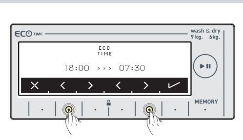
• You can adjust the Eco Time interval by touching the buttons of symbols  $\langle \rangle$ See page 60 to activate the Eco Time interval additional function.
