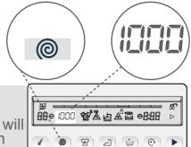
You can gradually reduce the revolution speed between cancel spinning (-) options through the maximum spin revolution of the programme selected by pressing revolution speed setting button.
