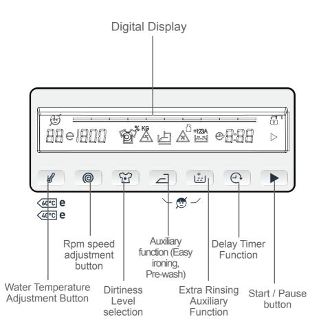
In the electronic display, you can see the washing water temperature of your machine, the wringing rpm, how long the machine has to finish washing, whether the door of your machine is locked or not, the auxiliary functions you have selected and the location of the programme you are running in your machine ( \_\_\_\_\_\_ ) among the washing sequence
