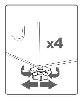
• Never put cardboard, wood or suchlike materials under your machine if you are intending to stabilize the distortions on the ground.
