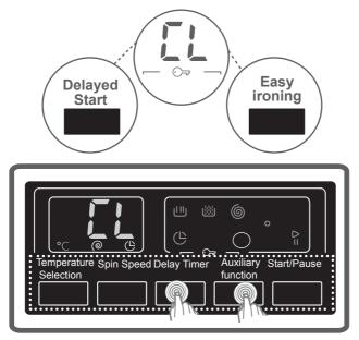
"CL" symbol will flash on the electronic display when activated.
