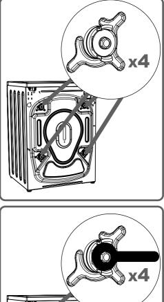
For this reason, transportation safety screws shall be loosened by being rotated in counter-clockwise using an appropriate wrench.
