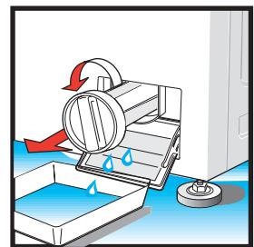
Removing the **drain pipe (F090)**:
